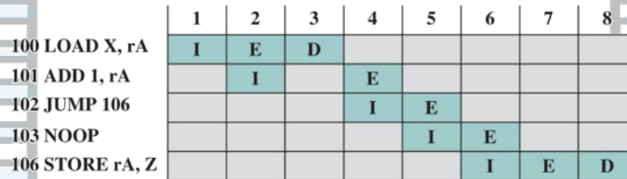
(b) RISC pipeline with inserted NOOP
